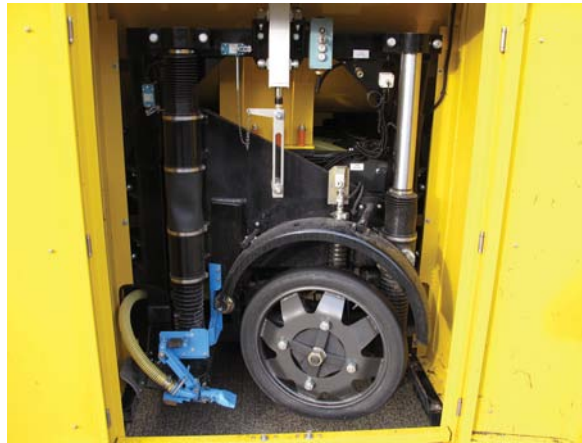
The SCRIM wheel is lowered on to the road surface at an angle of 20°
