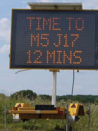
MVIS signs displaying temporary journey time technology
