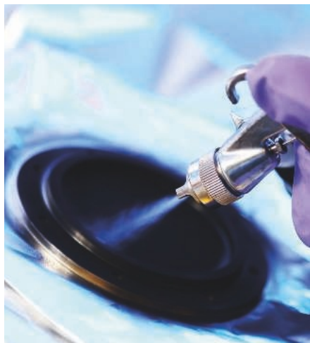
Vantablack S-VIS: An air applied coating with incredibly low reflectance
