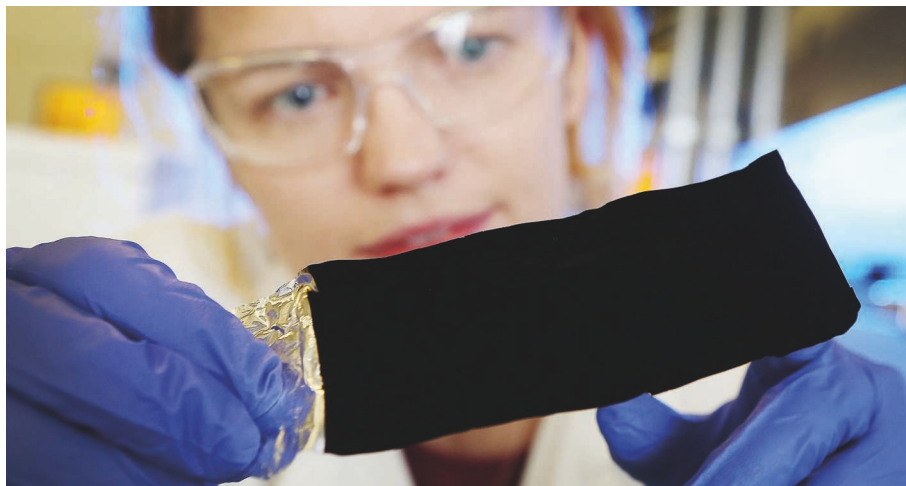
Vantablack S-VIS: An air applied coating with incredibly low reflectance
