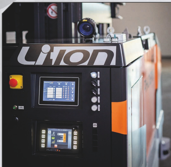
No driver's cab, but clearly laid out operating terminals.
