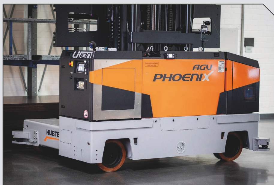
Also included: patented HX steering from Hubtex for a smooth changeover from longitudinal to transverse travel.
