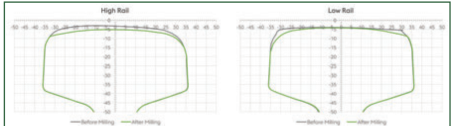
Figure 3: transversal rail profile before and after milling.
