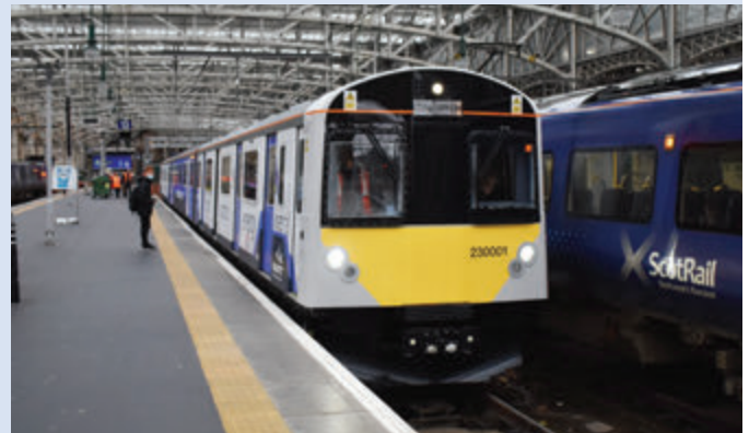
The converted former class 230 D-Train is equipped with six batteries.
