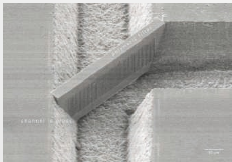
► Photonic crystals produced using the MPP technique, which is suitable for almost any geometric 3D structure. ►
