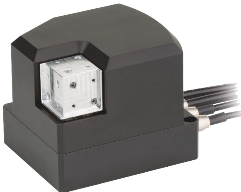
► The NanoCube 6-axis nanopositioning and scanning stage based on piezo flexure drives. Piezo flexure stages are available with up to six degrees of freedom (DOFs), allowing fast and highly precise scanning, positioning and alignment with virtually unlimited lifetime due to the non-wear and zero-friction design.► Image courtesy of PI.
