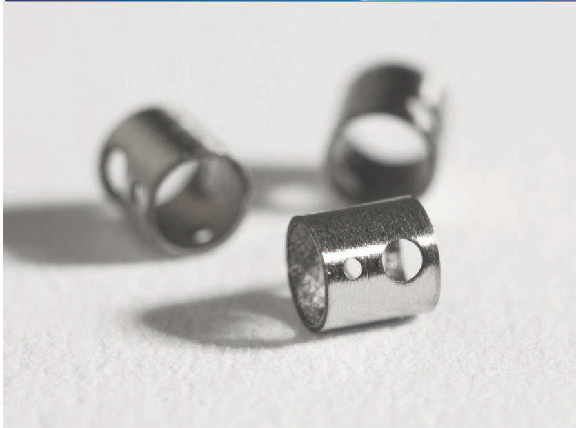
► Marker bands produced on the MLTC platform. These are attached to a catheter shaft via swaging or embedding to provide a high level of visibility under fluoroscopy. During surgery, the marker band serves as a shiny indicator of the exact location of the catheter tip inside the body. The MLTC small tube handling system is for 0.25 to 0.76 mm OD marker bands and the MLTC standard tube handling system is for larger than 0.76 mm OD marker bands. ►
