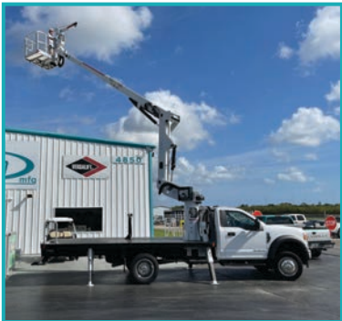
ATR-45N with 3' x 5' Aluminum Platform 1,000 lbs Material Handler. The ATR is offered in a 41, 45, 52, and 58 and all can be built on a Non-CDL truck
