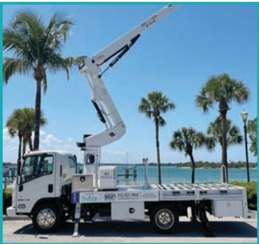
Stamm ATR-45N with 3' x 5' Aluminum Platform, 1,000 lbs Material Handler Mounted on a 19,500 GVWR Isuzu. Powered by the VanAir PowerFlex unit
