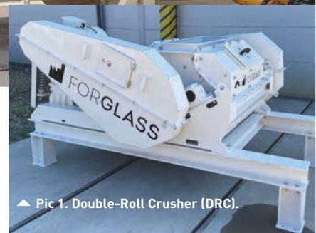
▲ Pic 1. Double-Roll Crusher (DRC).
