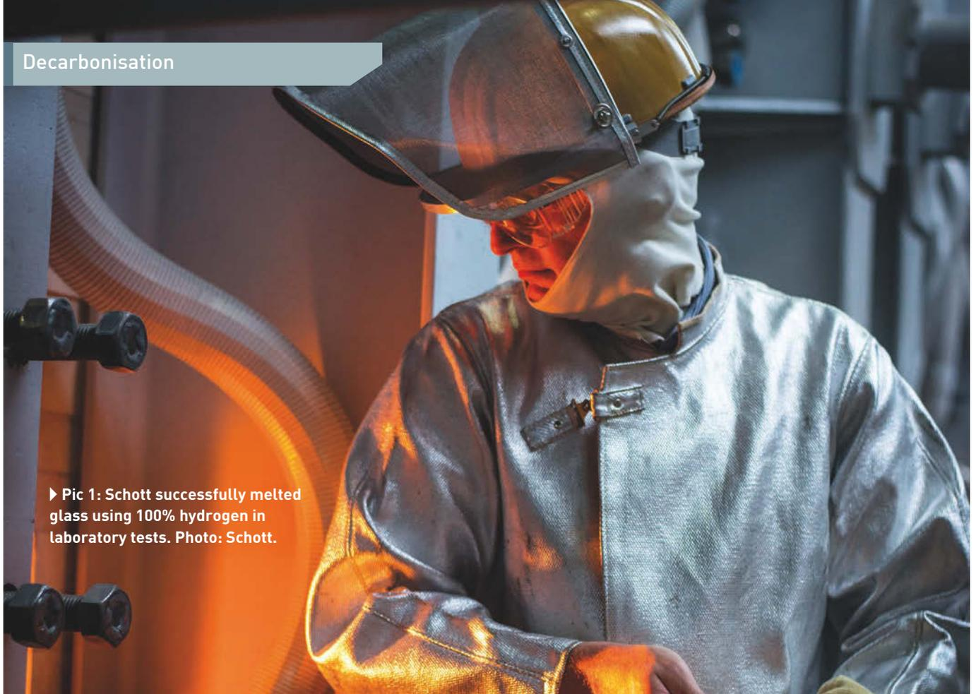
► **Pic 1: Schott successfully melted glass using 100% hydrogen in laboratory tests. Photo: Schott.**
