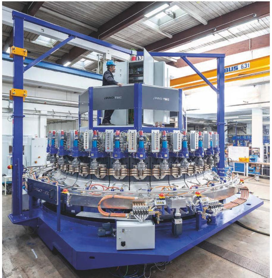
▲ Pic 1. The blowing machine from Iprotec has a modular design and can consist of up to 32 sections.
