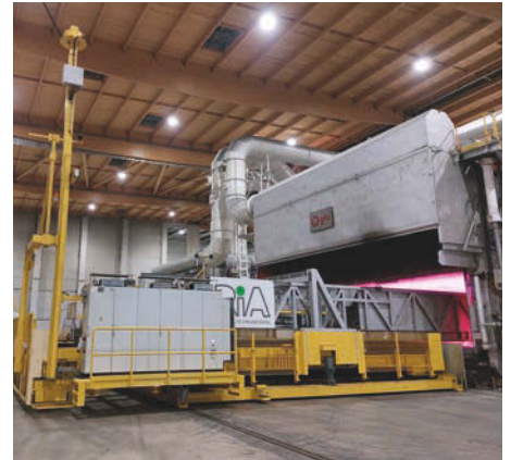
Image 2. Furnace Charging Machine, with its 60m³ Charging container
