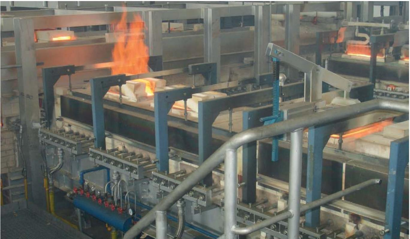
▲ Fig 1. Poor air/gas mixture setting: flames burst out of the chimney.
